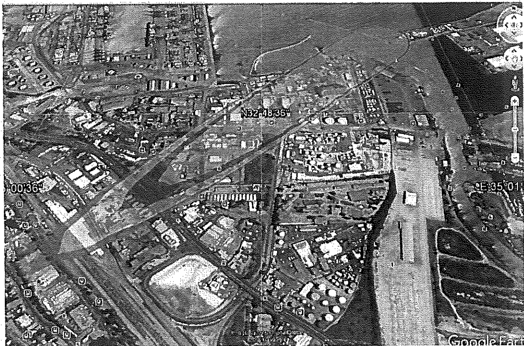
Figure 4; LCT Curve for Scenario 20: 2 Tank 2500 metric ton release with a 10 m/s wind; no buoyancy
